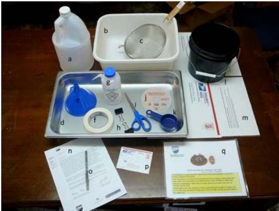
Figure 1: Reusable equipment needed for sampling apiaries. Materials include (a) 1 gallon bottle (to be filled with water), (b) wash tub, (c) strainer, (d) metal pan, (e) funnel, (f) clear binding tape, (g) squeeze bottle (to be filled with water), (h) binder clips, (i) scissors, (j) training video, (k) ¼ cup measuring cup, (l) bucket, (m) 3 large Priority Mail flat rate boxes, (n) letters explaining the purpose of this sampling (a copy of this should be given to cooperating beekeepers), (o) pen, (p) 3 preaddressed mailing labels, (q) Tropilaelaps information sheet.
